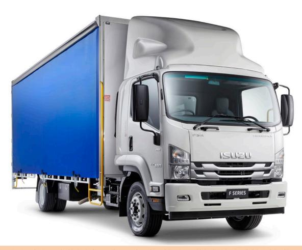
12 pallet (nominal) curtainside body / Easy glide curtains with quick release "Lightning" latches / Lightweight side gates /
